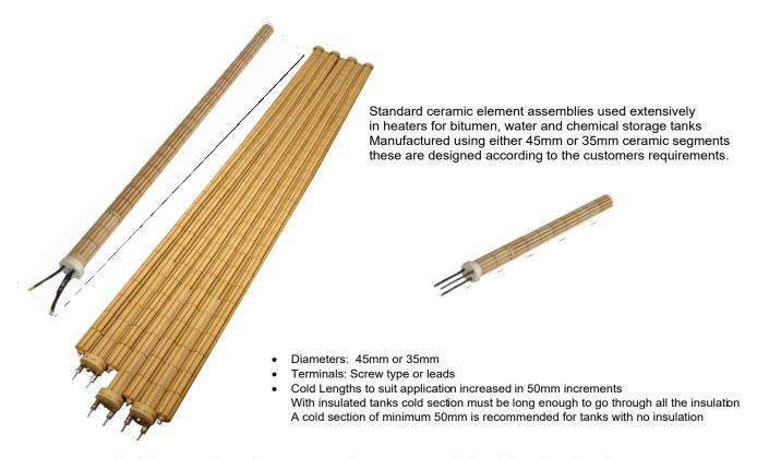
Lengths of elements can be as short as 200mm and up to 10000mm. The length depends on the rating watts density, and the length of cold and heated sections. The maximum standard construction is normally restricted to 6000mm If a longer length is required then an extended cold section can be fitted. See drawings below
